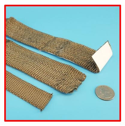
Basalt tapes do not fade or color change with heat exposure as do fiberglass tapes (plain, vermiculite coated or graphite coated). Basalt tapes also do not shed particles with vibration or movement as do coated fiberglass tapes.
