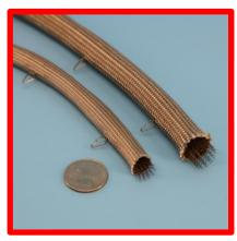
For applications such as commercial, industrial and scientific ovens and dryers, this gasket rope is easily installed by drilling a 1/8 inch hole into the door or frame on the equipment, and then inserting the self expanding clip into the hole.
