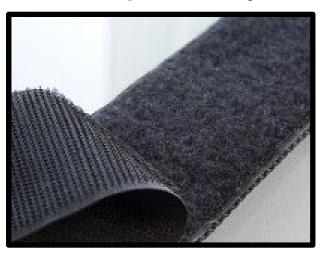
Nylon hook and loop closure with Urethane/Acrylic backcoat with Flame Retardant additive. 225°F / 107°C Continuous; 300°F / 148°C for up to 1 hour; 459°F / 237°C melting point. Color is black. Nomex<sup>®</sup> is rated -70°F to 350°F (-56°C to 176°C)
